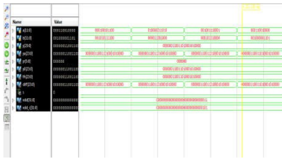
Fig 9: simulation result of ANT architecture when Row Bypassing multiplier is used.
